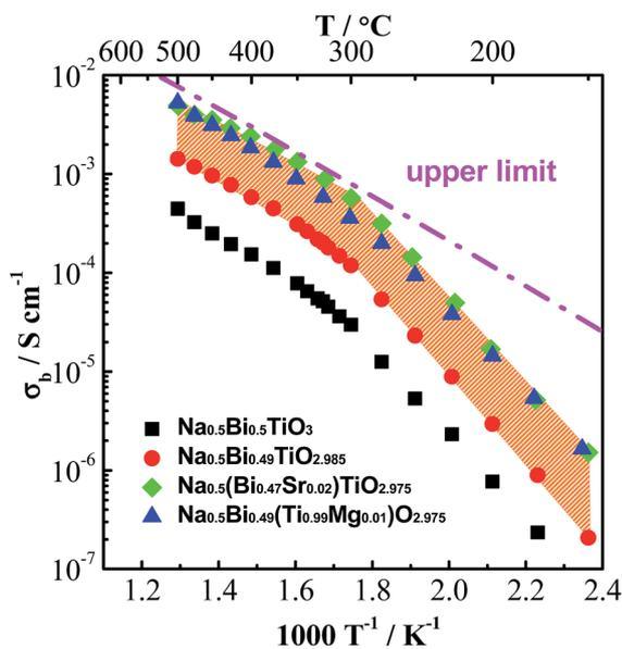
**Fig. 5** An Arrhenius plot of bulk conductivity,  $\sigma_b$ , for undoped and acceptor-doped NBT ceramics.<sup>41</sup> The dash-dot line represents the upper limit of  $\sigma_b$  based on the oxygen-vacancy diffusion coefficient predicted in ref. 45, see text.
