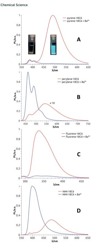
Fig. 5 Fluorescence spectra (CH<sub>3</sub>CN) of pyrene-18C6 (A), perylene-18C6 (B), fluorene-18C6 (C) and NMI-18C6 (D) without (red) and with (blue) Ba(ClO<sub>4</sub>)<sub>2</sub>. In panel A: picture of pyrene-18C6 without (left) and with (right) Ba<sup>2+</sup> under UV irradiation (366 nm).
