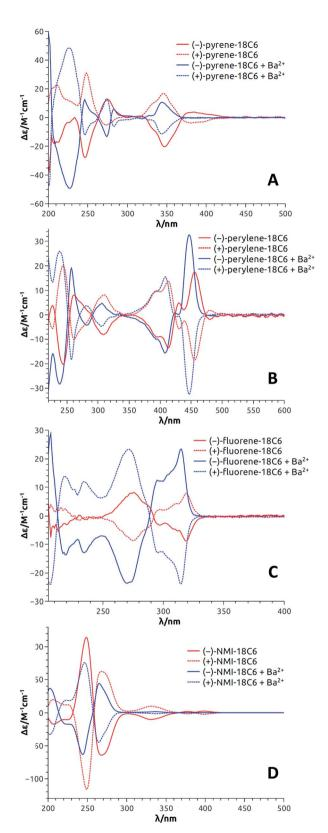
Fig. 4 ECD spectra (CH<sub>3</sub>CN) of both enantiomers of pyrene-18C6 (A), perylene-18C6 (B), fluorene-18C6 (C) and NMI-18C6 (D) without (red) and with (blue) Ba(ClO<sub>4</sub>)<sub>2</sub>.
