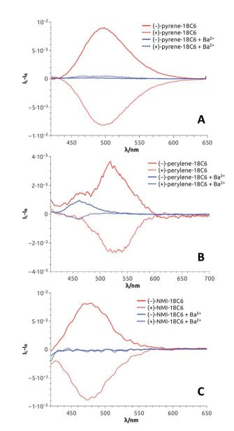
Fig. 7 CPL spectra (CH<sub>3</sub>CN) of both enantiomers of pyrene-18C6 (A), perylene-18C6 (B) and NMI-18C6 (C) without (red) and with (blue)  $Ba(ClO_4)_2$ .
