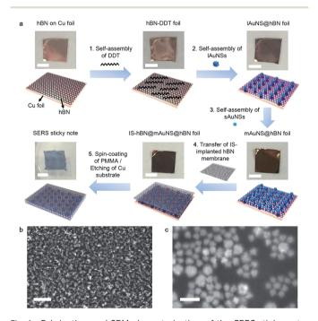
Fig. 1 Fabrication and SEM characterization of the SERS sticky note: (a) Optical images and schematic illustration of the step-by-step fabrication process of the SERS sticky note by self-assembly of DDT, lAuNSs and sAuNSs on hBN, encapsulation with IS-implanted hBN, spin-coating of PMMA, and etching of the Cu substrate. Scale bars: 2 mm. (b and c) SEM images of the SERS sticky note with scale bars of (b) 2 μm and (c) 200 nm.
