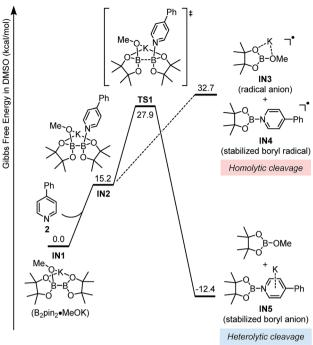
Fig. 5 Gibbs free energy ( $\Delta G_{solv\ 298\ K}$ ) profile for the homolytic and heterolytic cleavage pathways of diboron.
