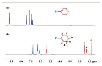
Fig. 1 <sup>1</sup>H-NMR spectra (400 MHz) of (a) 4-phenylpyridine and (b) reaction mixture shown in Scheme 2 at room temperature in THF.
