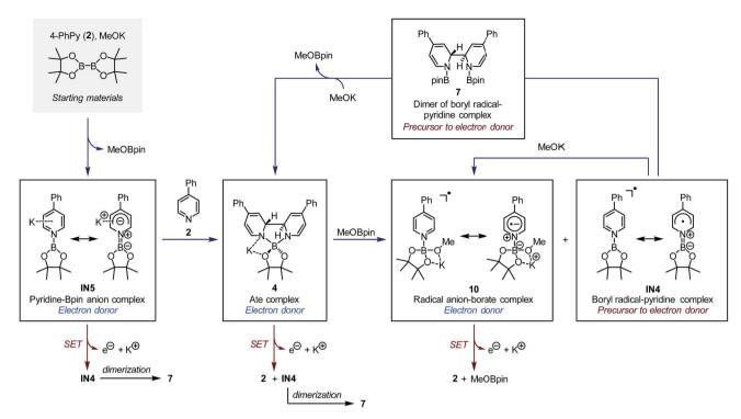
Fig. 7 Boryl-pyridine species involved in the reaction system and their interconversion. The blue arrows indicate the formation and interconversion between each species, while the red arrows indicate the single-electron transfer reaction of the electron donors.
