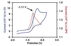
Fig. 2 CV and DPV plots of 2 mM complex  $4 \cdot \text{DME}$  in THF (0.1 M  $n\text{-Bu}_4\text{N}^+\text{PF}_6^-$  as the supporting electrolyte). The blue solid line: CV plot (scan rate = 0.1 V s<sup>-1</sup>); the red dashed line: DPV plot.
