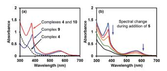
Fig. 4 (a) UV-vis spectra of the boryl-pyridine complexes in THF (red line: reaction mixture containing complexes 4 and 10; blue line: solution of complex 9 and 18-C-6; dashed line: solution of complex  $4 \cdot DME$ ). (b) UV-vis spectral change in the reaction mixture during the addition of iodoarene 5.
