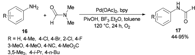
Scheme 6 Transamidation of aniline derivatives 16 with dimethylformamide.
