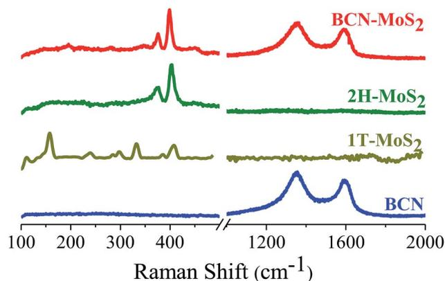
Fig. 17 Raman spectra of BCN, MoS<sub>2</sub> (1T), MoS<sub>2</sub> (2H) and BCN–MoS<sub>2</sub> composite.
