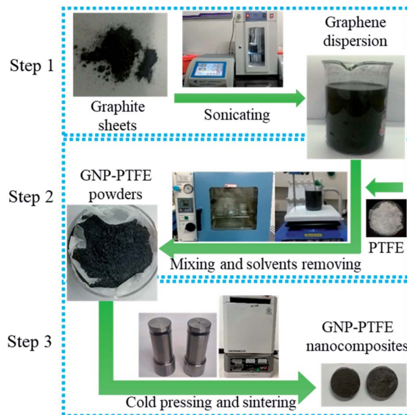
Fig. 1 Schematic of the method to fabricate the GNP–PTFE nanocomposites. Step 1: graphene dispersion was prepared by liquid phase exfoliation of graphite sheets in ethanol via tip sonication. Step 2: PTFE powders were added into the graphene dispersions and then fully mixed with GNPs while removing the ethanol using a heating magnetic stirrer for 6 h at 60 °C. Subsequently, the slurry was vacuum dried at 60 °C for 24 h to remove the residual ethanol in the GNP–PTFE powder. Step 3: the GNP–PTFE nanocomposites were fabricated by cold pressing with a mould and sintering.
