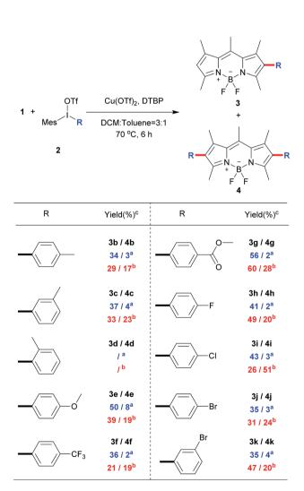
Scheme 3 Direct C-H arylation of BODIPY 1 with different diaryliodonium triflates.<sup>a</sup> Condition A: 0.8 equiv. of 2 was used; <sup>b</sup> condition B: 2.4 equiv. of 2 was used; cisolated yield.
