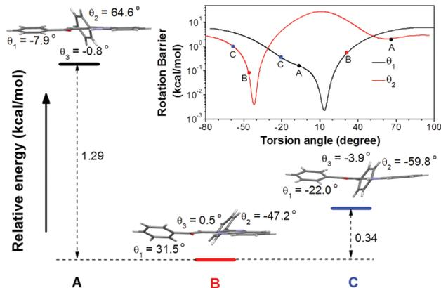
Fig. 5 Relative total energies of conformation A, B, and C. Inset: Rotational energy barrier obtained by rotating  $\theta_1$  and  $\theta_2$  in the optimized conformation.
