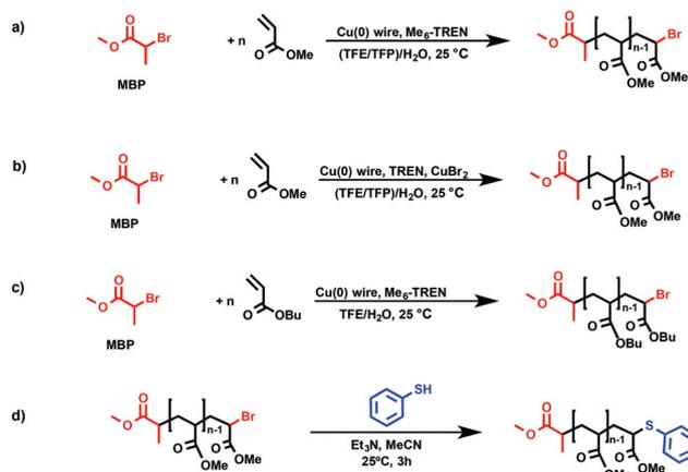
**Scheme 1** (a) Me<sub>6</sub>-TREN and (b) TREN-mediated SET-LRP of MA in binary mixtures of TFE or TFP with water in the presence of non-activated Cu(0) wire. (c) Me<sub>6</sub>-TREN-mediated SET-LRP of BA in binary mixtures of TFE with water in the presence of non-activated Cu(0) wire. (d) "thio-bromo click" modification of the corresponding PMA with thiophenol.
