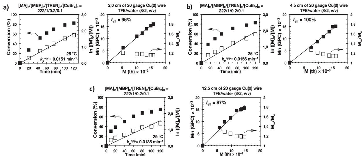
**Fig. 15** Kinetic plots, molecular weight and dispersity evolution for the SET-LRP of MA in TFE/water mixtures initiated with MBP and catalyzed by nonactivated Cu(0) wire at 25 °C. (a–c) TFE/water (8/2, v/v). The v/v ratio must be multiplied by 10 to obtain % solvent/% water. The value of v + v must be divided by 10 to obtain the total volume of solvents, 1 mL. Reaction conditions: MA = 1 mL, TFP + water = 0.5 mL,  $[MA]_0/[MBP]_0/[TREN]_0/[CuBr_2]_0 = 222/1/0.2/0.1$ .
