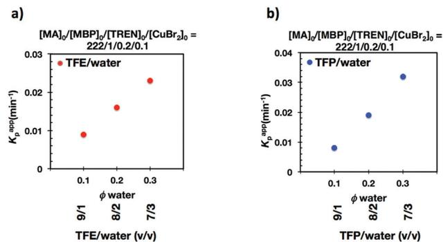
Fig. 9 The dependence of  $k_p^{\text{app}}$  with the volume fraction of water ( $\phi_{\text{H}_2\text{O}}$ ) on the SET-LRP of MA initiated with MBP mediated TREN/Cu(II)Br<sub>2</sub> and catalyzed by 4.5 cm of non-activated Cu(0) wire in (a) TFE/water and (b) TFP/water mixtures.
