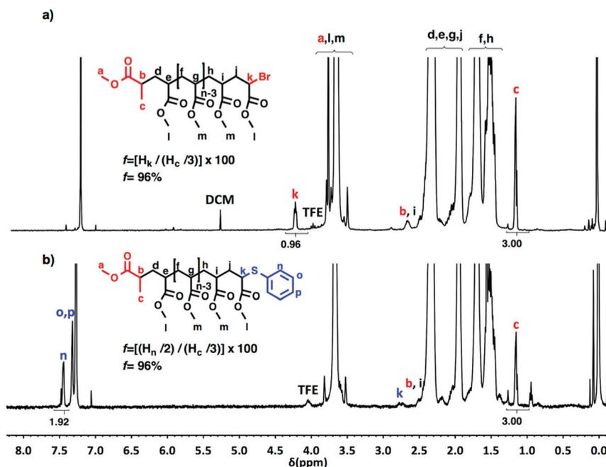
**Fig. 12**  $^1\text{H-NMR}$  (500 MHz) recorded in  $\text{CDCl}_3$ , of PMA-Br isolated at 88% conversion from SET-LRP of MA in TFE/water (8/2, v/v) mixtures initiated with MBP and catalyzed by nonactivated Cu(0) wire at 25 °C. (a) Before the “thio-bromo click” reaction. (b) After the “thio-bromo click” reaction. Reaction conditions: MA = 1 mL, TFE + water = 0.5 mL,  $[\text{MA}]_0/[\text{MBP}]_0/[\text{TREN}]_0/[\text{CuBr}_2]_0 = 50/1/0.2/0.1$ , 4.5 cm of 20 gauge Cu(0) wire.
