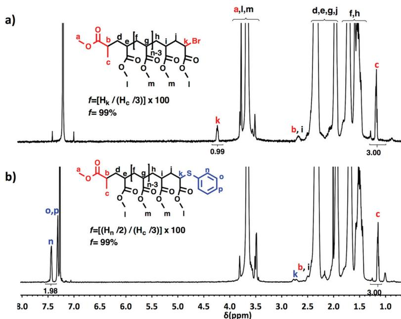
**Fig. 11**  $^1\text{H-NMR}$  (500 MHz) recorded in  $\text{CDCl}_3$ , of PMA-Br isolated at 86% conversion from SET-LRP of MA in TFE/water (8/2, v/v) mixtures initiated with MBP and catalyzed by nonactivated Cu(0) wire at 25 °C. (a) Before the “thio-bromo click” reaction. (b) After the “thio-bromo click” reaction. Reaction conditions: MA = 1 mL, TFE + water = 0.5 mL,  $[\text{MA}]_0/[\text{MBP}]_0/[\text{Me}_6\text{-TREN}]_0 = 50/1/0.1$ , 4.5 cm of 20 gauge Cu(0) wire.
