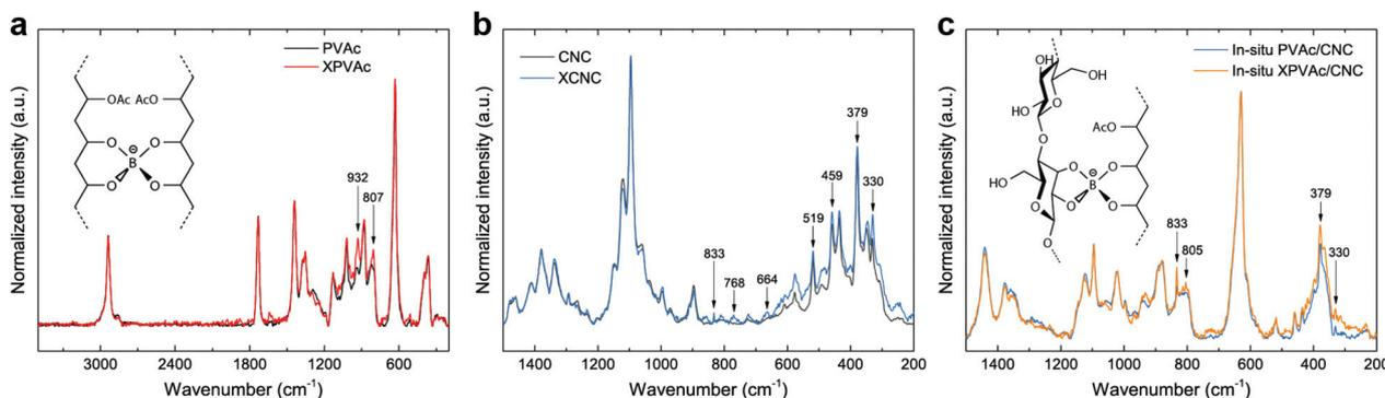
**Fig. 3** (a) Raman spectra of PVAc and XPVAc films in a spectral range of  $200\text{--}3500 \text{ cm}^{-1}$ , and the chemical structure of borax-crosslinked PVAc chains. (b) Raman spectra of CNCs and XCNCs in a spectral range of  $200\text{--}1500 \text{ cm}^{-1}$ . (c) Raman spectra of *in situ* PVAc/CNC and *in situ* XPVAc/CNC films (weight ratio of PVAc to CNCs is 80 : 20), and a possible chemical structure of borax-crosslinked PVAc–CNCs.
