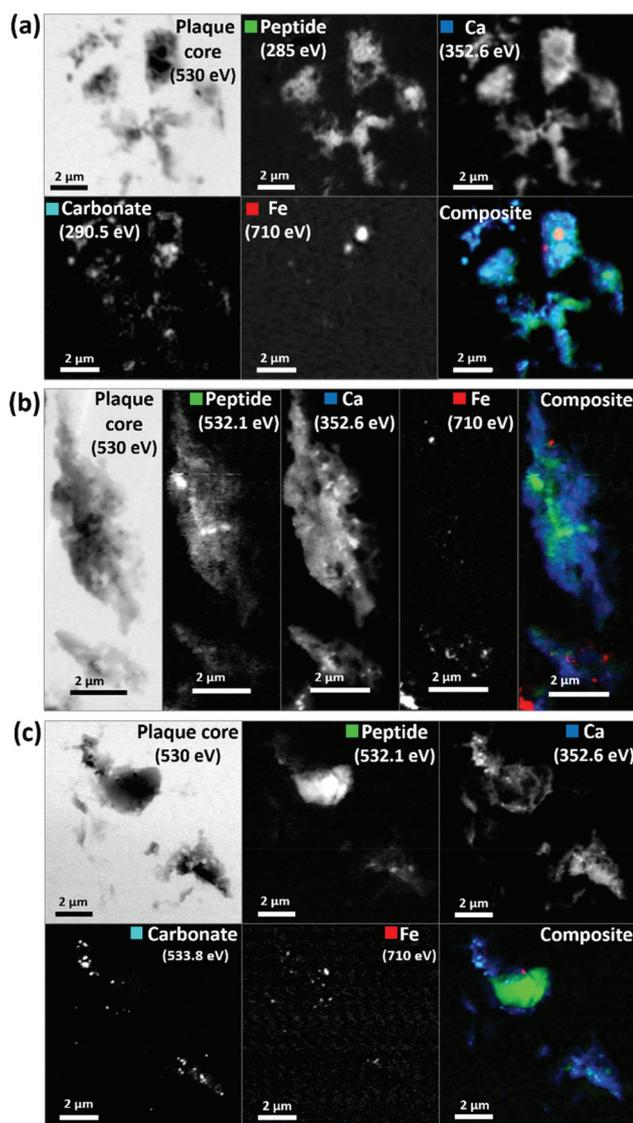
**Fig. 4** STXM images and speciation dependent contrast maps of amyloid plaque cores from case X (a), and case Y (b and c). The maps show the off-resonance (530 eV) image, oxygen K-edge peptide map (532 eV), calcium L-edge map (352 eV), oxygen K-edge carbonate map (533 eV), iron L-edge map (710 eV), and composite image displaying peptide (green), calcium (blue), carbonate (sky blue) and iron (red) content of the plaque core.
