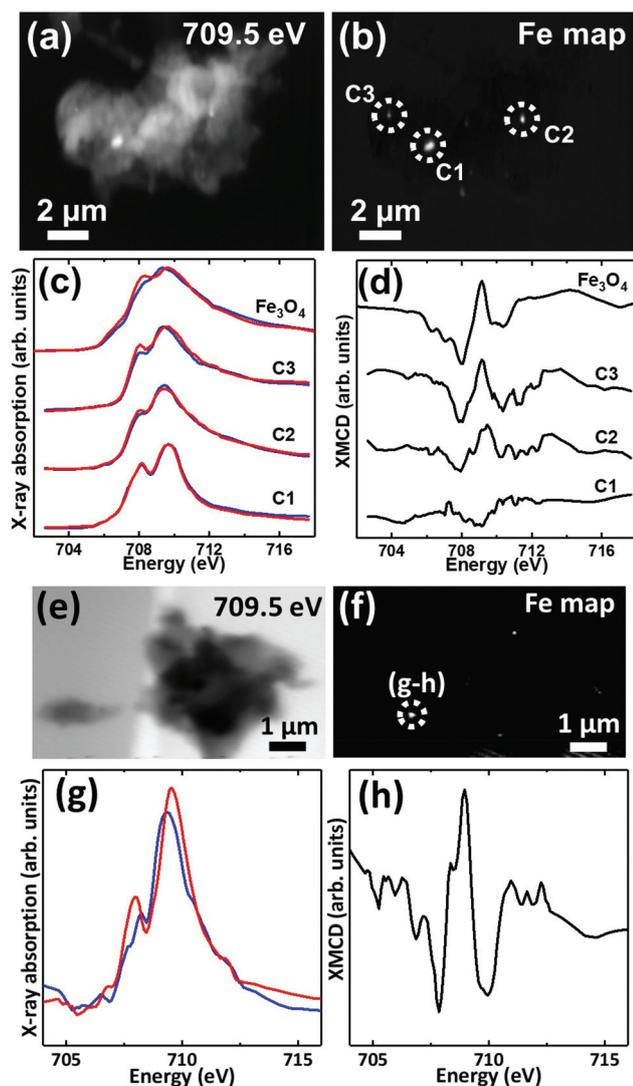
**Fig. 7** (a, e) X-ray microscopy images (b, f) iron  $L_3$  edge speciation maps (c, g) X-ray absorption spectra and (d, h) XMCD spectra from an APC of case X. Panels (c) and (g) show X-ray absorption spectra obtained using LCP (blue spectra) and RCP (red spectra). Panels (d) and (h) show the corresponding XMCD spectra created by subtracting the RCP spectra from the LCP spectra. All spectra were obtained in a magnetic field of  $\sim 150$  mT applied parallel to the incident X-ray beam.
