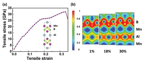
**Fig. 2** (a) The calculated stress–strain curve of  $\text{Mn}_2\text{AlB}_2$  with the ELF counter plots and (b) projected on the plane containing Mn and Al atoms under  $[0001]$  tensile strains of 1%, 18%, and 30%.
