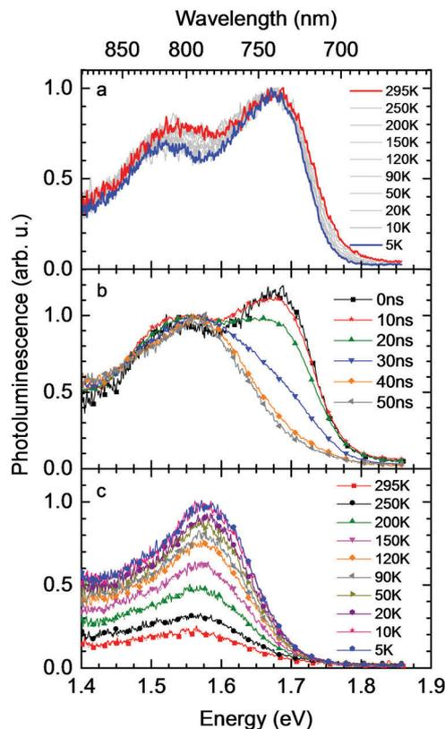
**Fig. 1** (a) Photoluminescence spectra of a MeLPPP:PCBM blend recorded at different temperatures with zero delay and 10 ns gate width, normalized to maximum intensity (b) emission spectra of a MeLPPP:PCBM blend at room temperature with different delay times and 10 ns integration time, normalized to about 1.55 eV (c) evolution of the emission spectrum with temperature 90 ns after excitation. While the 5 K spectrum is normalized to unity, all spectra show the correct relative intensity.
