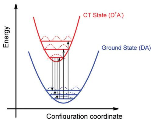
**Fig. 6** Schematic illustration of the energy surface of  $S_0$  and CT state. The general configuration coordinate reflects mostly the distance and orientation between donor and acceptor. Note the steeper potential and thus higher vibrational frequencies in the excited state.
