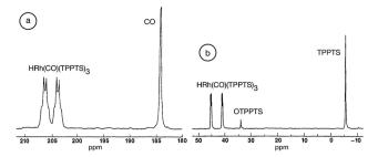
Fig. 1 <sup>13</sup>C NMR (a) and <sup>31</sup>P NMR (b) spectra of HRh(<sup>13</sup>CO)(TPPTS)<sub>3</sub> in the presence of a 3 molar excess of TPPTS under a 200 bar pressure of  $^{13}CO$ :  $H_2 = 1:1$  in  $D_2O$ . Modified with permission from ref. 59. Copyright of Springer (1989).
