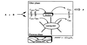
Fig. 2 Original drawing of the fluorous biphase concept for the catalytic conversion of substrates A and B to product P. Adapted from ref. 93. Copyright of The American Association for the Advancement of Science (1994)
