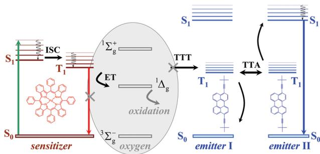
**Fig. 1** Simplified energetic scheme of the triplet–triplet annihilation upconversion process in an oxygen contaminated environment, containing singlet oxygen scavenging moieties. Insets: Structure of the sensitizer (PdTBP) and emitter (BDP); SOS – singlet oxygen scavenger.
