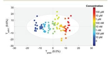
Fig. 6 OPLS analysis score plot. Each point represents one spectrum in the subspace generated by the predictive ( $T_{\rm pred}$ ) and first orthogonal (T<sub>orth</sub>) components. The different concentrations are indicated with colors (color scale on the right).
