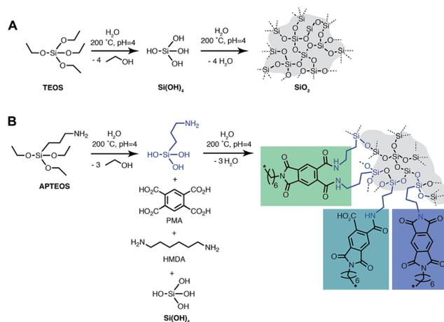
Fig. 4 Reaction equation of SiO<sub>2</sub> and PI6/SiO<sub>2</sub> co-condensation. (A) Hydrothermal hydrolysis and condensation sequence from TEOS to SiO<sub>2</sub>. (B) Co-condensation of PI6 and SiO<sub>2</sub> in the presence of the compatibilizer APTES; possible linkages (1,2-diamide, amic acid; and imide) are shown.
