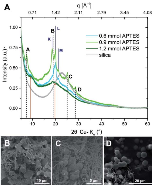
Fig. 6 PI6/ $\text{SiO}_2$  prepared from PMA, HMDA, APTES and TEOS. (A) Diffractograms of the hybrids prepared at different  $n_{\text{APTES}}$ , and diffractogram of hydrothermally synthesized  $\text{SiO}_2$  for comparison (grey). (B)–(D) SEM images of the corresponding hybrids at  $n_{\text{APTES}} = 0.6$  mmol (B),  $n_{\text{APTES}} = 0.9$  mmol, and  $n_{\text{APTES}} = 1.2$  mmol.
