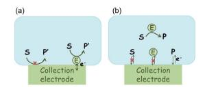
Fig. 1 Illustration of two possible enzyme detection methods via the nano-impact technique. (a) The enzyme collides with the electrode with which it undergoes direct electron transfer. (b) The catalytic reaction of the enzyme occurs in solution and the product is detected electrochemically
