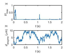
Fig. 6 Example of a simulated random walk current (a) and the corresponding pathway in the solution (b). The space, in which the enzyme moves freely, ranges from 5 nm to 10  $\mu$ m. Other simulation parameters are the same as applied in Fig. 5.
