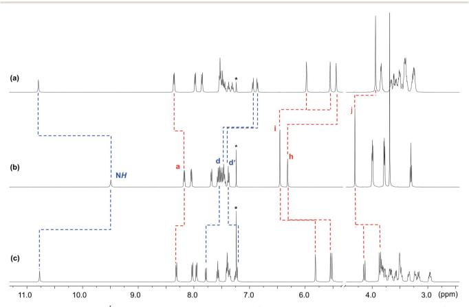
Fig. 2 Comparison of the partial  $^1$ H NMR spectra (500 MHz, CDCl<sub>3</sub>) of (a) suit[1] ane **6a**, (b) an equimolar solution of **1** and **7** and (c) suit[1] ane **6b** (\* = CHCl<sub>3</sub>). Labelling scheme is shown in Scheme 2 for **1** and **7**.
