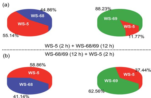
Fig. 8 Pie charts showing the adsorption proportions of dyes WS-5, WS-68 and WS-69 in the cosensitization strategy on 16  $\mu\text{m}$   $\text{TiO}_2$  films.
