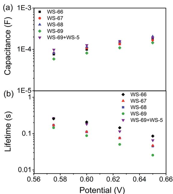
**Fig. 7** TiO<sub>2</sub> capacitance (a) and electron lifetime (b) as a function of potential based on WS-66, WS-67, WS-68, WS-69 and cosensitization of WS-5 with WS-69.
