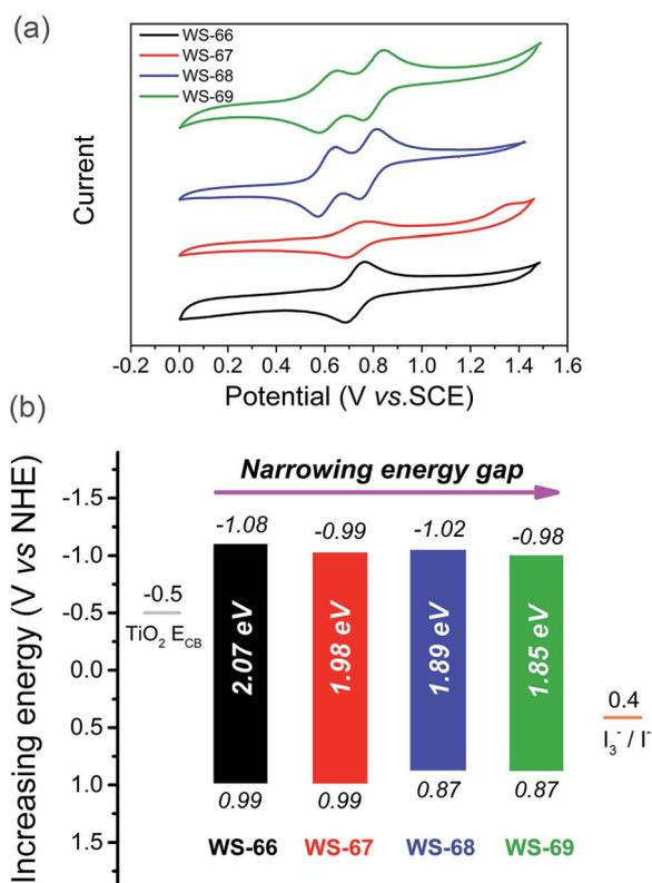
Fig. 3 Cyclic voltammograms of dyes WS-66, WS-67, WS-68 and WS-69 measured in CH<sub>2</sub>Cl<sub>2</sub> (a), LUMO (above the coloured bar) and HOMO (under the coloured bar) values, and energy band gaps of dyes WS-66, WS-67, WS-68 and WS-69 (b).
