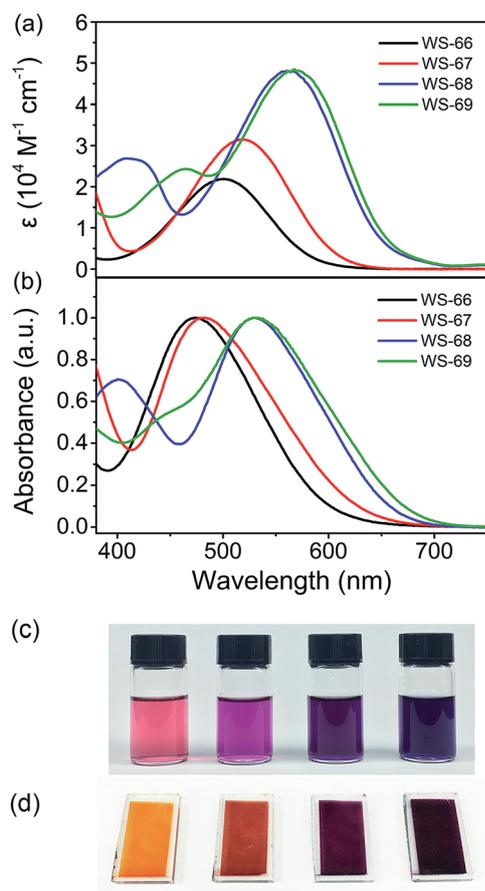
Fig. 2 Absorption spectra of dyes **WS-66**, **WS-67**, **WS-68** and **WS-69** in  $\text{CH}_2\text{Cl}_2$  (a) and on  $3 \mu\text{m}$   $\text{TiO}_2$  films (b). Photographs of dyes **WS-66**, **WS-67**, **WS-68** and **WS-69** (from left to right) in solution (c) and on  $\text{TiO}_2$  films (d).
