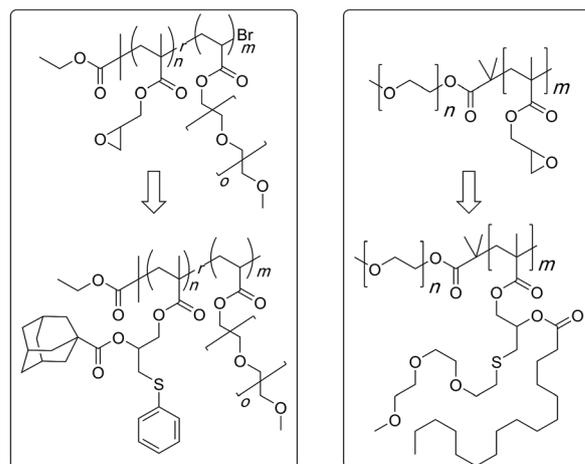
**Scheme 9** Application of the thiol-epoxy and esterification reactions-based sequential modifications strategy to prepare poly(ethylene glycol)-based doubly modified water soluble copolymers.
