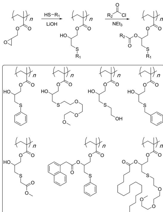
**Scheme 8** First application of the thiol-based ring-opening reaction for modification of the PGMA scaffold. In this study, bi-functional structures were also synthesised through esterification of the generated secondary hydroxyl groups. The top shows the general synthetic scheme and the bottom shows various singly and doubly functionalised structures.
