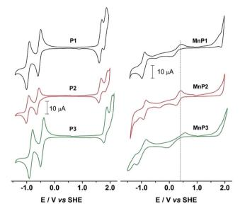
Fig. 2 Cyclic voltammograms of  $H_2P$  and MnP in dichloromethane containing 0.1 mol  $L^{-1}$  TBAPF<sub>6</sub>. Scan rate at 100 mV s<sup>-1</sup>. Initial anodic scan.
