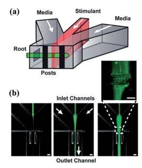
Fig. 5 The schematic diagram of a gradient generator and the obtained fluorescence images. (a) A Y-shape junction with three inlets. (b) Three fluorescence images obtained by the junction in (a) with different flow rates. The total flow rate is 200  $\mu L$  min $^{-1}$  and the flow rate ratios of the three inlets are (from left to right): 10:1:10,5:1:5,2:1:2 (left: middle: right stream). (Reproduced from ref. 89 with permission from the Royal Society of Chemistry).
