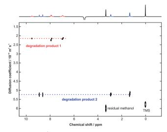
Fig. 4  $\,$  500 MHz  $^{1}$ H DOSY spectrum, with the least attenuated 1D spectrum shown at the top, acquired after 17 h of monitoring of a sample containing 24 mM voriconazole, and 48 mM NaOH in CD<sub>3</sub>OH at 10 °C.
