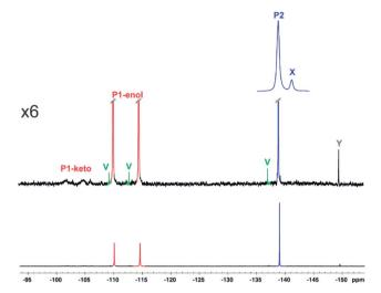
Fig. 6 Expansion of  $^{19}$ F NMR spectrum acquired after 24 h with the same sample as Fig. 4.
