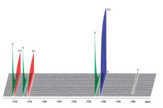
Fig. 3 <sup>19</sup>F NMR spectra during a 17 h alkaline stress test, showing the consumption of voriconazole (V), the formation of major degradation products 1 (P1) and 2 (P2), and minor degradation products X and Y. Spectra are shown at half hour intervals
