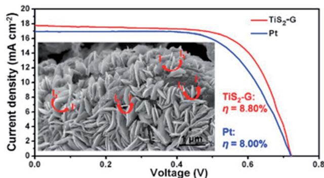
Fig. 12 A comparison of photocurrent density-voltage ( $J-V$ ) curves of DSSCs having TiS<sub>2</sub>-graphene hybrid and Pt counter electrodes. Reprinted with permission from ref. 199, X. Meng, C. Yu, B. Lu, J. Yang and J. Qiu, dual integration system endowing two-dimensional titanium disulfide with enhanced triiodide reduction performance in dye-sensitized solar cells. *Nano Energy*, 2016, 22, 59-69. Copyright© Elsevier.
