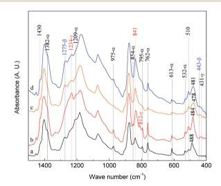
Fig. 5 FTIR spectra of electrospun membranes from 12 wt% PVDF under different flow rates and ratios of NMP and acetone ( $V_{NMP}$ /  $V_{\text{acetone}}$ ): curve 'a' (black) for 60  $\mu$ L h<sup>-1</sup> and  $V_{\text{NMP}}/V_{\text{acetone}} = 8/2$ ; curve b' (red) for 2000 μL  $h^{-1}$  and  $V_{NMP}/V_{acetone} = 8/2$ ; curve 'c' (orange) for 60  $\mu$ L h $^{-1}$  and  $V_{NMP}/V_{acetone}=7/3$ ; curve 'd' (blue) for 500  $\mu$ L h $^{-1}$  and  $V_{\rm NMP}/V_{\rm acetone} = 7/3.$
