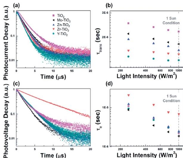
Fig. 19 (a and c) Photocurrent and photovoltage decay of devices employing the  $\text{TiO}_2$  ETL incorporated with different acetylacetonate-based additives and (b and d) the related carrier transport lifetime and electron lifetime. Intensity is shown in log scale and 1 sun condition is equivalent to  $1000 \text{ W m}^{-2}$ .
