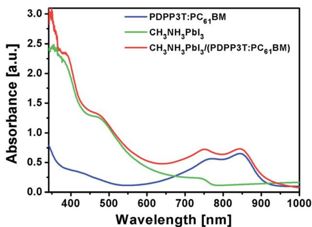
Fig. 26 Comparison of absorption spectra for PDPP3T-PC<sub>61</sub>BM (1 : 2) blend film, CH<sub>3</sub>NH<sub>3</sub>PbI<sub>3</sub> film, and CH<sub>3</sub>NH<sub>3</sub>PbI<sub>3</sub>/(PDPP3T-PC<sub>61</sub>BM) (1 : 2) bilayer film.<sup>133</sup>
