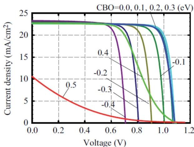
Fig. 2  $J$ - $V$  curves of perovskite solar cells with different CBO values of buffer/absorber interface. Here, the VBO of the absorber/HTM interface was set to 0 and the interface defect density of IDL 1 was set to  $10^{16} \text{ cm}^{-3}$ .<sup>67</sup>
