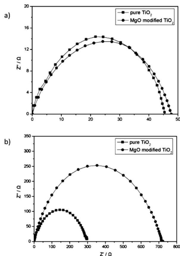
Fig. 10 EIS of PSC with and without MgO coating under (a) light illumination and (b) dark conditions.<sup>104</sup>
