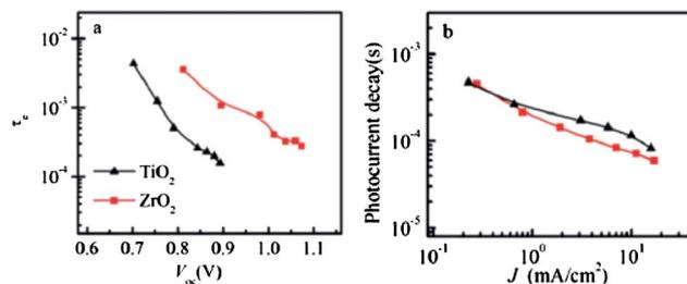
Fig. 7 (a) Electron lifetime as a function of open circuit voltage in Spiro-OMeTAD/CH<sub>3</sub>NH<sub>3</sub>PbI<sub>3</sub>/ZrO<sub>2</sub> (or TiO<sub>2</sub>) solar cells. (b)<sup>84</sup> Photocurrent transient decay occurs as a function of short-circuit current in Spiro-OMeTAD/CH<sub>3</sub>NH<sub>3</sub>PbI<sub>3</sub>/ZrO<sub>2</sub> (or TiO<sub>2</sub>) solar cells.<sup>84</sup>
