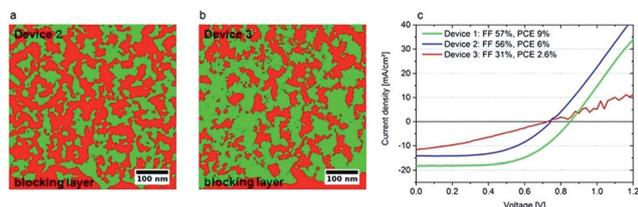
Fig. 16 Correlation between morphology and device characteristics. (a) Device 2 exhibits a compact and well-connected TiO<sub>2</sub> network. (b) The TiO<sub>2</sub> in device 3 is a much finer grained structure (very small and unconnected red domains). (c) *J*-*V* characteristics of the devices. The higher fill factors of devices 1 and 2 can be correlated to the well-connected TiO<sub>2</sub> network and hence better electron transport properties.<sup>66</sup>
