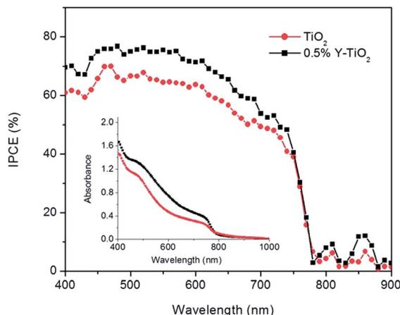
Fig. 12 Incident photon-to-electron conversion efficiency spectra of devices based on 0.5% Y-TiO<sub>2</sub> (black) and TiO<sub>2</sub> (red). The inset shows the UV-Vis absorbance spectra of 0.5% Y-TiO<sub>2</sub>/CH<sub>3</sub>NH<sub>3</sub>PbI<sub>3</sub> and TiO<sub>2</sub>/CH<sub>3</sub>NH<sub>3</sub>PbI<sub>3</sub> electrodes.<sup>34</sup>
