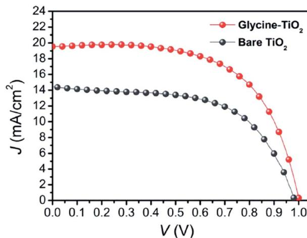
Fig. 27  $J$ - $V$  curves of the best perovskite solar cells with bare TiO<sub>2</sub> (dark gray curve) and glycine-treated TiO<sub>2</sub> (red curve).<sup>137</sup>
