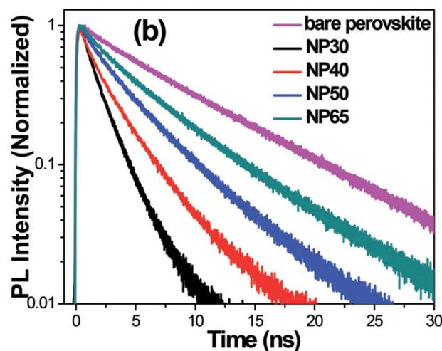
Fig. 4 TR-PL decays of bare  $\text{CH}_3\text{NH}_3\text{PbI}_3$  deposited on Pyrex glass and the  $\text{FTO}/\text{TiO}_2/\text{CH}_3\text{NH}_3\text{PbI}_3$  devices employing NP30, NP40, NP50, and NP65. It can be seen clearly that the TR-PL decay is accelerated with decrease in the size of  $\text{TiO}_2$  NPs. The time resolution of the TR-PL measurement was  $\sim 190 \text{ ps}$ .<sup>77</sup>
