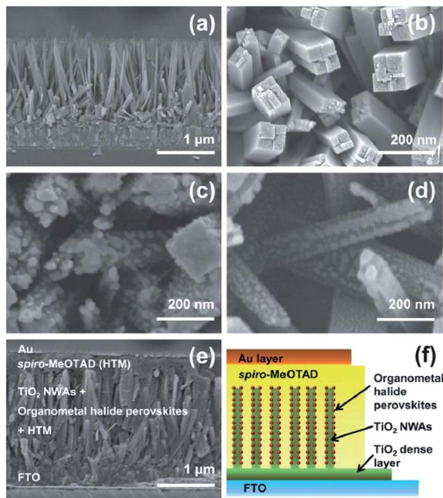
Fig. 17 Cross-sectional (a) and top (b) view SEM images of TiO<sub>2</sub> nanowire arrays (NWAs) synthesized on FTO substrates. SEM images of CH<sub>3</sub>NH<sub>3</sub>PbI<sub>2</sub>Br (c) and CH<sub>3</sub>NH<sub>3</sub>PbI<sub>3</sub> (d) spin-coated on TiO<sub>2</sub> NWAs. (e) Cross-sectional SEM image of the TiO<sub>2</sub> NWAs/perovskite sensitizer/spiro-MeOTAD hybrid photovoltaic cell. (f) Schematic illustration of the hybrid solar cell.
