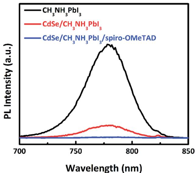
Fig. 8 The PL spectra of  $\text{CH}_3\text{NH}_3\text{PbI}_3$ ,  $\text{CdSe}/\text{CH}_3\text{NH}_3\text{PbI}_3$ ,  $\text{CdSe}/\text{CH}_3\text{NH}_3\text{PbI}_3/\text{Spiro-OMeTAD}$  on glass substrates. The excited wavelength is 600 nm.<sup>78</sup>
