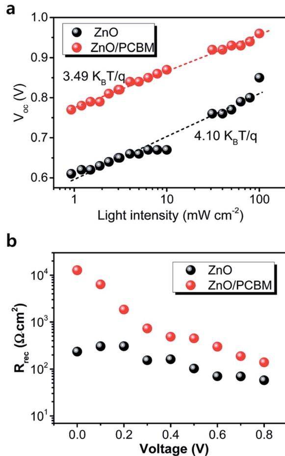
Fig. 20 (a) Light-intensity dependence of the  $V_{oc}$  of the perovskite solar cells with ZnO and ZnO/PCBM. The lines represent the best fits to the data, for which the slope is indicated. (b) Recombination resistance extracted from IS characterization of the perovskite solar cells.<sup>128</sup>
