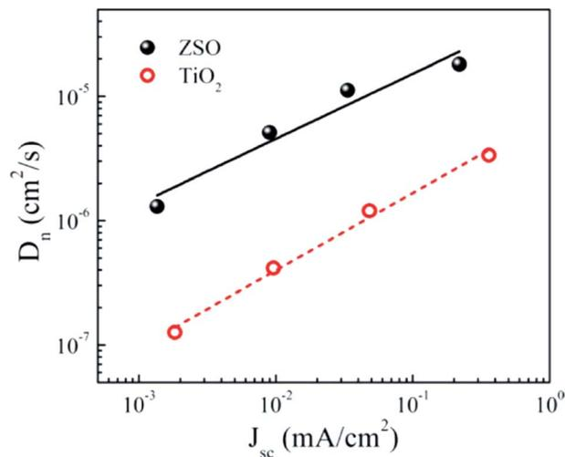
Fig. 18 Electron diffusion coefficients of the ZSO-based perovskite solar cell with the highest conversion efficiency. Electron diffusion coefficients of a TiO<sub>2</sub>-based perovskite solar cell with similar thickness (~300 nm) and conversion efficiency (~7%) are also presented for a comparison.<sup>118</sup>
