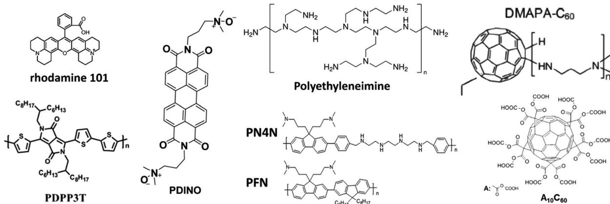
Fig. 24 Different polymer additives used in organic electron transport layers.<sup>131</sup>
