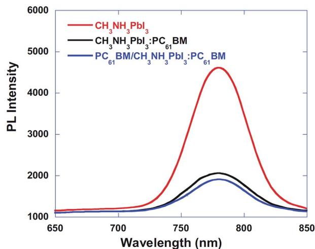
Fig. 21 Photoluminescence (PL) spectra of the pristine  $\text{CH}_3\text{NH}_3\text{-PbI}_3$ ,  $\text{CH}_3\text{NH}_3\text{PbI}_3:\text{PC}_{61}\text{BM}$ , and  $\text{PC}_{61}\text{BM}/\text{CH}_3\text{NH}_3\text{PbI}_3:\text{PC}_{61}\text{BM}$  thin films.<sup>124</sup>
