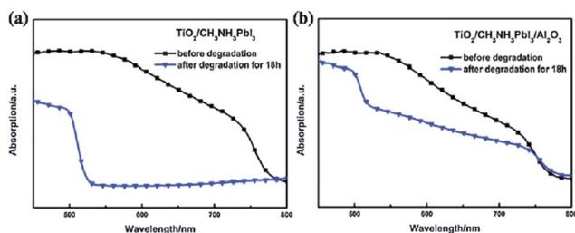
Fig. 6 UV-Vis spectra of sensitized films. (a) Film of TiO<sub>2</sub>/CH<sub>3</sub>NH<sub>3</sub>PbI<sub>3</sub> before and after degradation, (b) Film of TiO<sub>2</sub>/CH<sub>3</sub>NH<sub>3</sub>PbI<sub>3</sub>/Al<sub>2</sub>O<sub>3</sub> before and after degradation. The degradation time is 18 h.<sup>85</sup>
