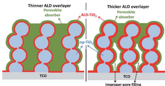
Fig. 9 Block diagrams of mesoscopic photoanodes with thinner (left) and thicker (right) ALD  $\text{TiO}_2$  overlayer (red) deposited on the mesoporous nanoparticle  $\text{TiO}_2$  (light blue) films. The np- $\text{TiO}_2$ -ALD  $\text{TiO}_2$  film is infiltrated with  $\text{CH}_3\text{NH}_3\text{PbI}_3$  absorber (green). For thicker ALD  $\text{TiO}_2$  overlayers, the pore diameter is reduced and improper pore filling of the perovskite absorber is highlighted (right).<sup>98</sup>
