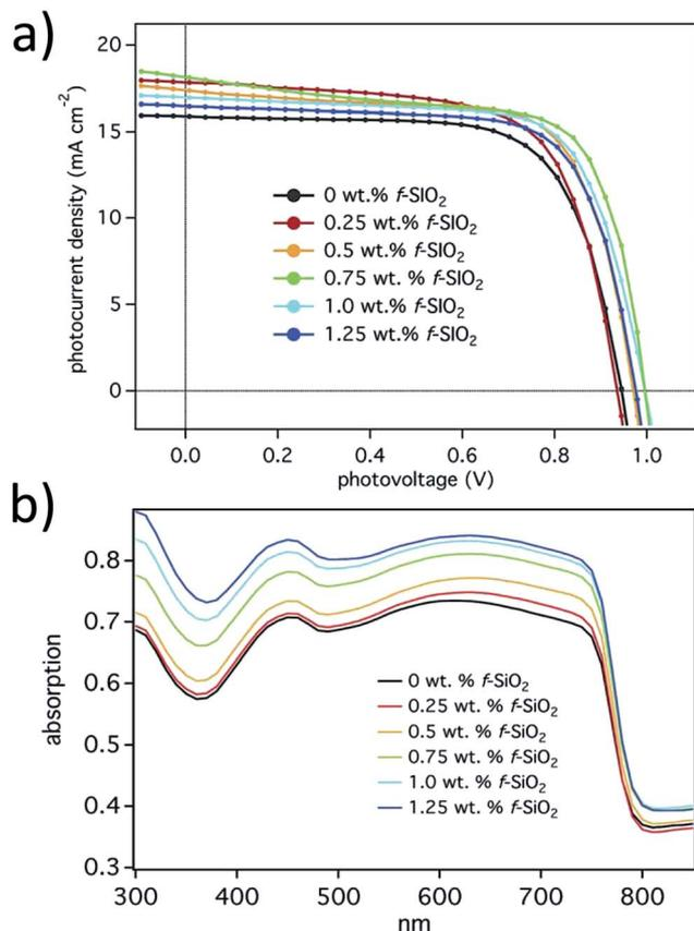
Fig. 29 (a)  $I$ - $V$  curves of best performing devices for each  $f\text{-SiO}_2$  wt%; (b) UV-Vis reflectance spectra of perovskite films with varying  $f\text{-SiO}_2$  wt% loadings.<sup>140</sup>
