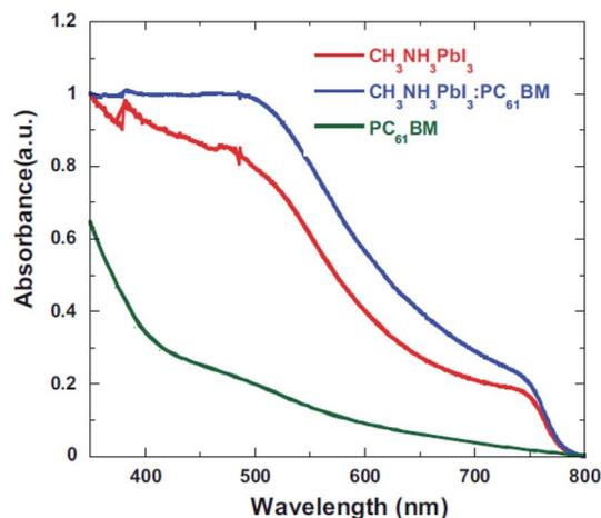
Fig. 22 Absorption spectroscopy of  $\text{CH}_3\text{NH}_3\text{PbI}_3$ ,  $\text{CH}_3\text{NH}_3\text{PbI}_3:\text{PC}_{61}\text{BM}$ , and  $\text{PC}_{61}\text{BM}/\text{CH}_3\text{NH}_3\text{PbI}_3:\text{PC}_{61}\text{BM}$  thin films.<sup>124</sup>
