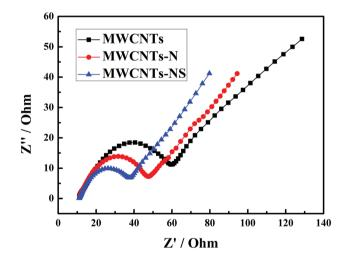
Fig. 4 Electrochemical impedance spectroscopy of glassy carbon electrodes modified by different MWCNTs samples in 1.0 mol  $\rm L^{-1}$  VOSO $_4$  + 3.0 mol  $\rm L^{-1}$   $\rm H_2SO_4$  at open-circuit voltage.
