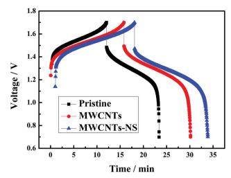
Fig. 6 The  $10^{th}$  charge–discharge curves of the cell using the MWCNTs samples as a catalyst in the positive side at a current density of 50 mA cm<sup>-2</sup>.
