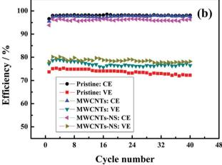
Fig. 7 The discharge capacity (a) and efficiency (b) of the cells using different MWCNTs samples as a function of cycle number at the current density of 50 mA  $\rm cm^{-2}$ .
