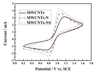
Fig. 3 Cyclic voltammetry curves of glass carbon electrodes modified by different MWCNTs samples at the scan rate of 20 mV s $^{-1}$  in a 2.0 mol L $^{-1}$  VOSO $_4$  + 3.0 mol L $^{-1}$  H $_2$ SO $_4$  electrolyte solution.
