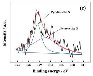
Fig. 2  $\,$  XPS survey of MWCNTs-NS (a) and high resolution XPS of  $S_{2p}$  (b) and  $N_{1s}$  (c).
