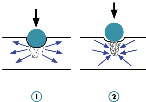
Fig. 2 Deformation profile of (1) non-auxetic material and (2) auxetic material.<sup>25</sup>
