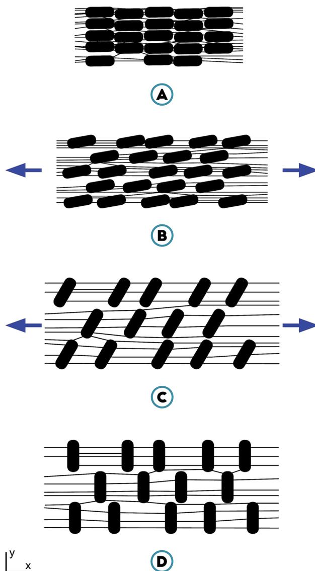
Fig. 6 Structural changes observed in microporous PTFE undergoing tensile loading in the  $x$ -direction.<sup>90</sup> (A) Nearly fully densified state. (B) Tension in fibrils causes particle displacement. (C) Rotation of the disc-shaped particles. (D) Fully expanded condition.<sup>89</sup>
