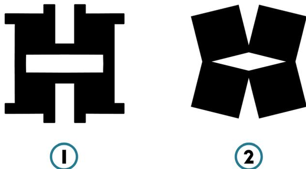
Fig. 11 Cellular plates with (1) rectangular perforations and (2) rhomboidal perforations.<sup>118</sup>
