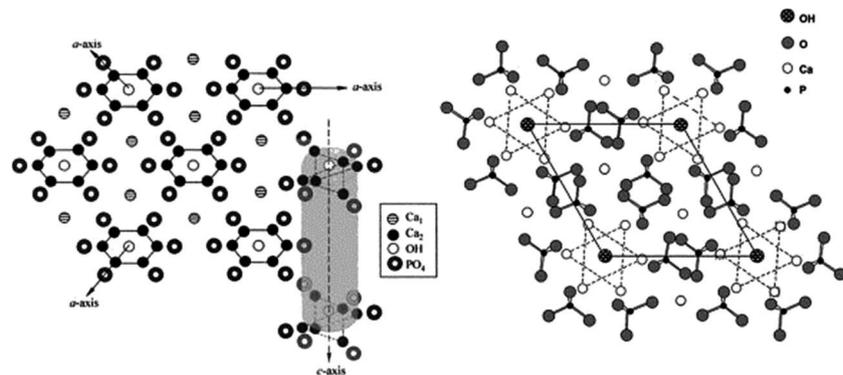
Fig. 3 Crystal structure of HA showing the  $c$ -axis perpendicular to 3  $a$ -axes lying at  $120^\circ$  of each other (left), and projection of the HA structure on the 001 plane (right) (this figure was reproduced with permission from John Wiley and Sons).<sup>4</sup>
