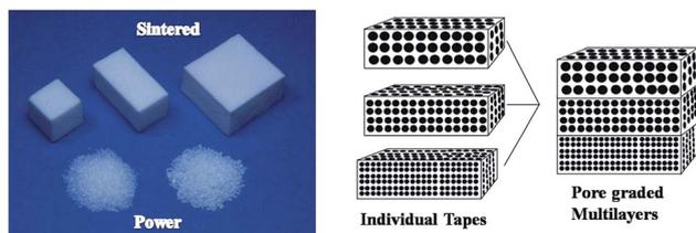
Fig. 13 Example of sintered HA used as an artificial bone substitute (reproduced with permission from MDPI)<sup>146</sup> and graded porous HA materials using tape-casting and lamination (reproduced with permission from MDPI).<sup>147</sup>
