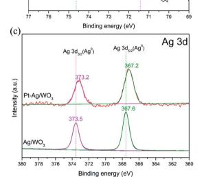
Fig. 5 XPS spectra of (a) W 4f and (b) Pt 4f and (c) Ag 3d high-resolution spectra for the different as-prepared samples.
