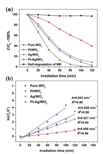
Fig. 7 (a) Photocatalytic degradation ratio of MB solution in the presence of pure  $WO_3$ ,  $Pt/WO_3$ ,  $Pt/WO_3$  and  $Pt-Ag/WO_3$  thin films. (b) Plots of  $In(C_0/C)$  versus irradiation time.
