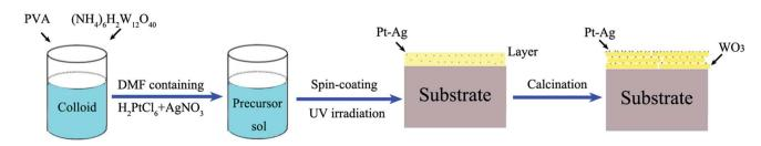
Scheme 1 Schematic illustration of the preparation process of Pt-Ag/WO<sub>3</sub> thin films.
