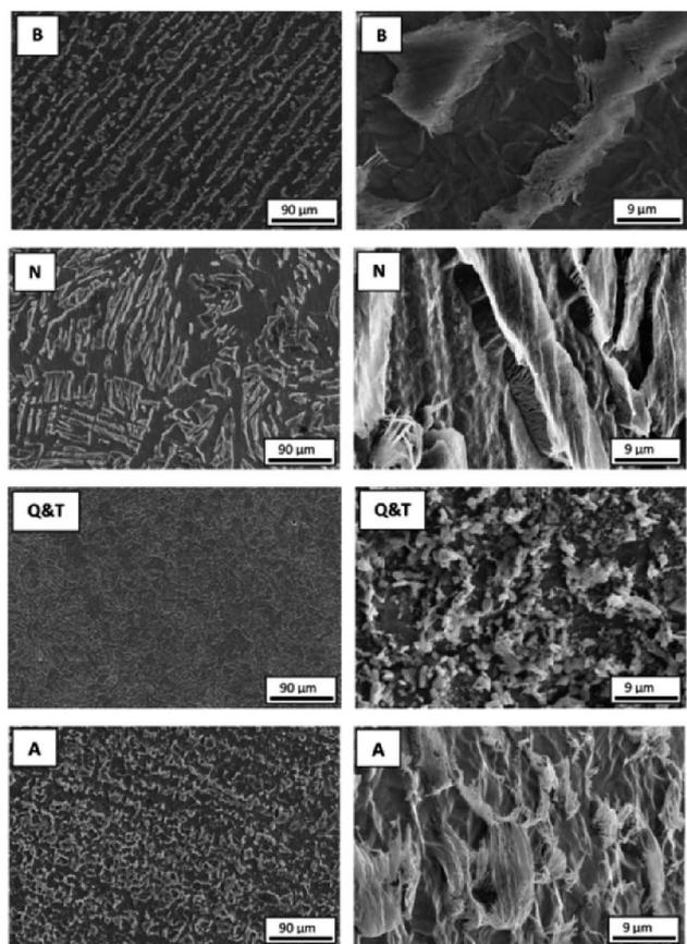
Fig. 13 Appearance of morphological differences after corrosion (with hold time of 6 h in 0.5 M NaCl solution saturated with CO<sub>2</sub>) of banded (B), normalized (N), quenched and tempered (Q & T) and annealed (A) steels shown by SEM morphological images with two different magnifications.<sup>100</sup> Reprinted with permission from ref. 100. Copyright 2015, Elsevier B. V.
