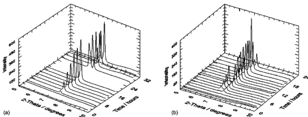
Fig. 10 *In situ* SR-GIXRD results for a polished mild steel electrode immersed in 3% (w/v) NaCl saturated with high purity carbon dioxide (at atmospheric pressure (adjusted to pH 4.75)) without (a) and with acetic acid (b) 200 mg L<sup>-1</sup> of acetic acid.<sup>90</sup> Reprinted with permission from ref. 90. Copyright 2007, Elsevier B. V.
