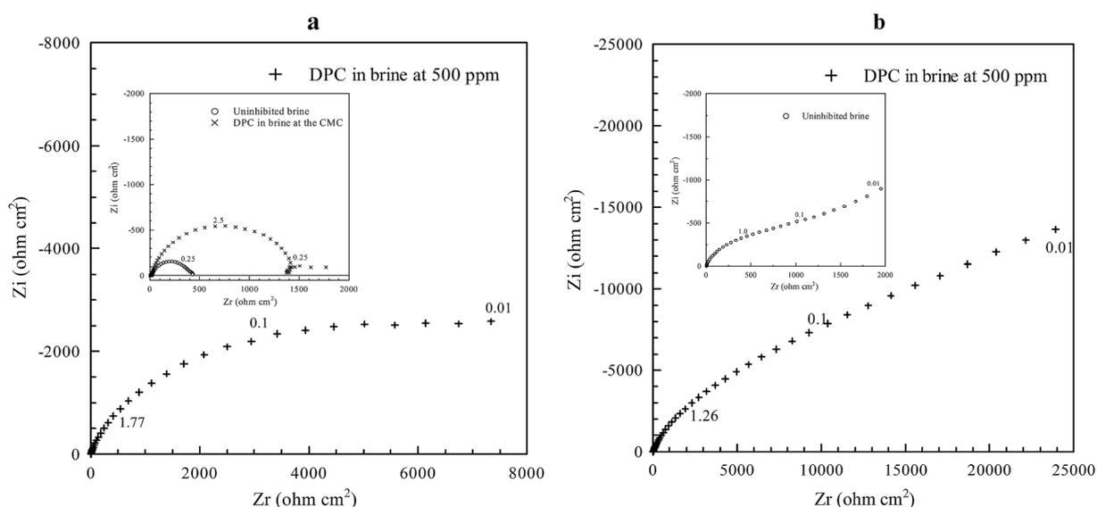
Fig. 8 Electrochemical impedance spectroscopy Nyquist plots for (a) CO<sub>2</sub>-saturated brine with 500 ppm DPC (inset: uninhibited brine and DPC at the CMC) and (b) N<sub>2</sub>-saturated brine with 500 ppm DPC for carbon steel after 4 h immersion.<sup>83</sup> Reprinted with permission from ref. 83. Copyright 2014, American Chemical Society.
