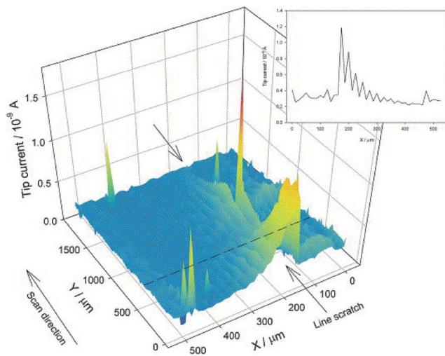
Fig. 19 SECM image of tinplate with a line scratch immersed in 10 mM  $\text{H}_2\text{SO}_4$ . The current increase above the scratch shows the oxidation of  $\text{Fe}^{2+}$  to  $\text{Fe}^{3+}$ .  $E_{\text{tip}} = +600$  mV,  $E_{\text{sample}} = \text{OCP}$  (about 520 mV), SECM Pt tip radius: 10  $\mu\text{m}$ .<sup>168</sup> Reprinted with permission from ref. 168. Copyright 2006, Elsevier B. V.
