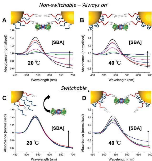
**Fig. 2** UV-Vis traces of different nanoparticle formulations in presence of serial dilution of SBA ( $10\text{--}1\ \mu\text{g mL}^{-1}$ ) after 30 minutes incubation. All particles (60 nm) had [pHEA<sub>15</sub>-Gal]:[pNIPAM<sub>x</sub>] 8:2. pNIPAM<sub>25</sub> at 20 °C (A) and 40 °C (B); pNIPAM<sub>50</sub> at 20 °C (C) and 40 °C (D). An increase in Abs<sub>700</sub> and decrease in Abs<sub>540</sub> is indicative of binding. All curves normalise so Abs<sub>450</sub> = 1.
