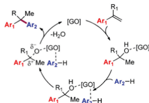
Scheme 7 Proposed mechanism for the GO-catalyzed alkylation of arenes. Reproduced from ref. 74 with permission from American Chemical Society, copyright 2017.
