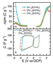
**Fig. 4** Electrochemical stability window determination. (a) difference between  $q_{\rm charge}$  and  $q_{\rm discharge}$ . (b) CV at determined limit voltage for positive and negative sweep for the ILs [Im<sub>1,4</sub>][C(CN)<sub>3</sub>] (blue), [Pyr<sub>1,4</sub>][C(CN)<sub>3</sub>] (red) and [Pip<sub>1,4</sub>][C(CN)<sub>3</sub>] (green).
