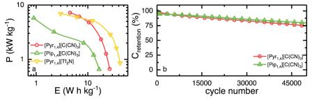
Fig. 7 (a) Ragone plot of EDLCs using  $[Pyr_{1,4}][C(CN)_3]$  (at 2.9 V, red),  $[Pip_{1,4}][C(CN)_3]$  (at 3.0 V, green) and  $[Pyr_{1,4}][Tf_2N]$  (at 3.5 V, yellow) for comparison. Values were calculated from the galvanostatic charge-discharge experiments at different specific currents, considering the electrodes active mass. (b) long-term stability of EDLCs containing  $[Pyr_{14}][C(CN)_3]$  and  $[Pip_{14}][C(CN)_3]$  operating at 2.0 A  $g^{-1}$ , from 0 V to the operating voltage.
