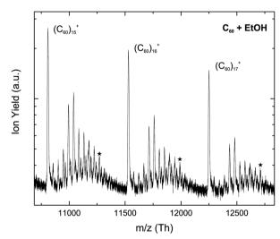
Fig. 3 A section of the mass spectrum measured upon electron ionization of helium droplets doped with  $C_{60}$  and ethanol in the region of the  $(C_{60})_{16}^+$  cluster. The most pronounced peaks, apart from those from bare  $(C_{60})_n^+$  ions, correspond to the attachment of 4 and 5 ethanol molecules to the  $(C_{60})_n^+$  cluster. The peaks labelled with an asterisk are for a  $(C_{60})_n^+$  ion with 10 attached ethanol molecules.
