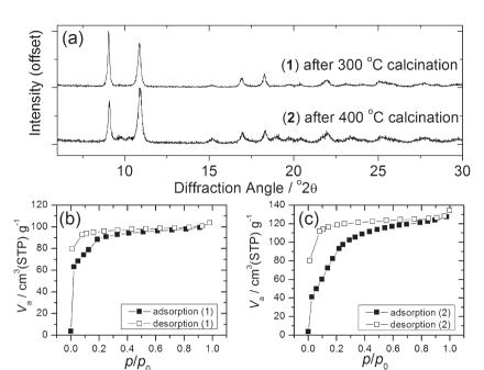
Fig. 6 (a) XRD of Yb<sub>2</sub>(BDC)<sub>3</sub> prepared from (1) and (2) and (b) and (c) BET nitrogen adsorption isotherms of each phase.
