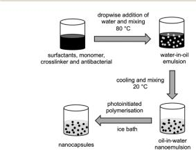
Fig. 2 Synthesis of nanocapsules by phase inversion temperature method.
