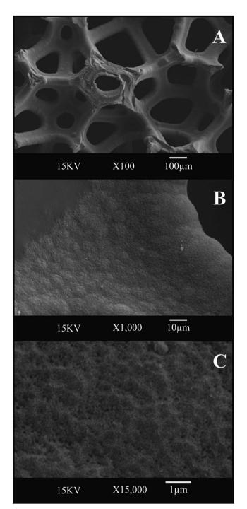
Fig. 1 SEM images of the freestanding 3D GNR foam at an increasingly higher magnification, (A)  $\times$ 100, (B)  $\times$ 1000 and (C)  $\times$ 15 000.
