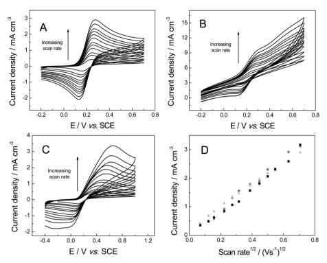
Fig. 4 Cyclic voltammetric profiles recorded in 1 mM potassium ferrocyanide(II) in pH 7 PBS (with 0.1 M KCl), utilising the freestanding 3D GNR (A), 3D PTGR (B) and RVC (C) foam electrodes. (D) Depicts the analysis of voltammetric peak height vs. square-root of the applied scan rate at the freestanding 3D GNR (light grey triangles), 3D PTGR (black squares) and RVC (dark grey circles) foam electrodes.
