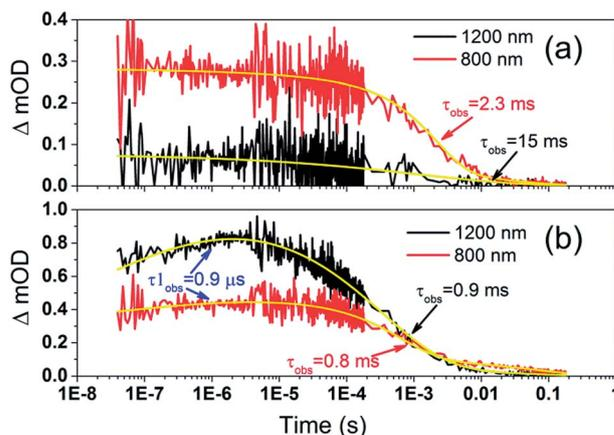
Fig. 6 Transient absorption decays and fitted functions of (a)  $\text{TiO}_2$ -Por and (b)  $\text{TiO}_2$ -Por-(Cb-TPA) with the inert electrolyte  $\text{I}_0$  (532 nm, 45–50  $\mu\text{J cm}^{-2}$  per pulse; repetition rate 1 Hz).
