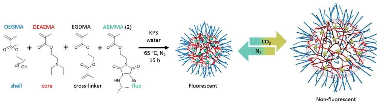
**Scheme 2** Synthesis of particles (**8**) *via* emulsion polymerization in water at 65 °C and the reversible particle response upon CO<sub>2</sub> and N<sub>2</sub> bubbling.
