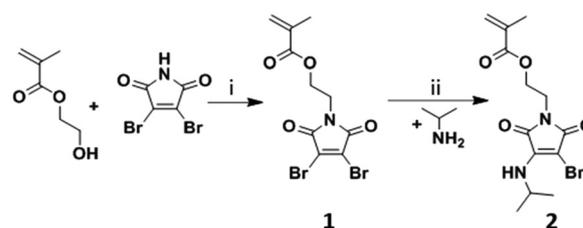
**Scheme 1** Synthesis of the ABMMA monomer (**2**). Conditions: (i) PPh<sub>3</sub>, DIAD, 2,2-dimethylpropan-1-ol in THF; (ii) Na<sub>2</sub>CO<sub>3</sub> in THF.
