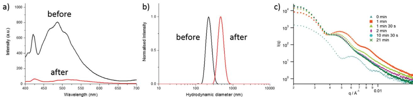
**Fig. 2** (a) Fluorescence emission spectra of particles **8** before and after the first CO<sub>2</sub> bubbling, (b) DLS of particles **8** before and after the first CO<sub>2</sub> bubbling, (c) *in situ* size monitoring of particles **3** by SAXS over 21 min of CO<sub>2</sub> bubbling.
