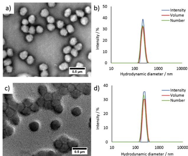
**Fig. 1** (a) TEM image of particles **4**, (b) DLS analysis of particles **4**, (c) TEM image of particles **8**, (d) DLS analysis of particles **8**. TEM grids were stained with an aqueous solution of uranyl acetate, see ESI† for more details.<sup>35</sup>
