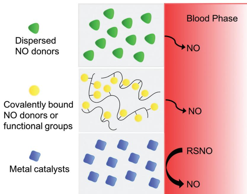
**Fig. 7** Three different strategies to fabricate of polymer surfaces that release or generate NO, including physical dispersion of NO donor into polymeric matrix, covalently bound NO donor functionalities onto polymer backbone, or NO generation from endogenous RSNO species in blood by metal catalysts embedded in or covalently bound to the surface of the polymer.
