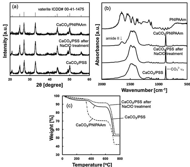
Fig. 2 XRD patterns (a), FT-IR spectra (b), and TG curves (c) of the CaCO<sub>3</sub>-polymer composite microspheres.
