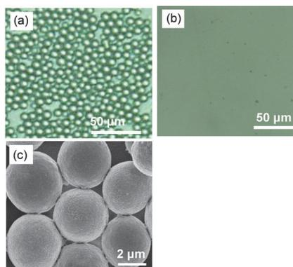
Fig. 4 Optical micrographs (a, b) and SEM image (c) of the CaCO<sub>3</sub>-PNIPAAm composites on an alkyl-modified glass substrate after washing in water by sonication at 60 °C (a, c) and 25 °C (b).
