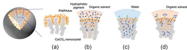
Fig. 8 Schematic illustration of a trap–release mechanism of the hydrophobic pigment on the  $\text{CaCO}_3$ –PNIPAAm composites (a). The hydrophobic pigment is trapped by PNIPAAm with swelling by the organic medium above LCST (b). The pigment is kept in the nanopores in water below LCST (c). The pigment is released into the organic phase with swelling by the organic medium above LCST (d).
