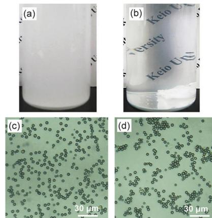
Fig. 3 Macroscopic and microscopic images of the dispersion of CaCO<sub>3</sub>-PNIPAAm composites in water at 25 °C (a, c) and 60 °C (b, d).
