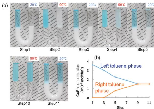
Fig. 7 Photographs of a toluene–water–toluene system containing the  $\text{CaCO}_3$ –PNIPAAm composites and CuPh in a U-tube (a). CuPh was transported with the  $\text{CaCO}_3$ –PNIPAAm composites from the left toluene phase into the right toluene phase through the water phase by a swing in temperature. The CuPh concentration of the left and right toluene phases changed with the cycle of temperature (b).
