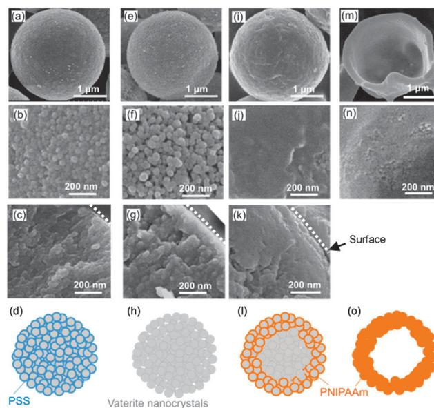
Fig. 1 SEM images and schematic illustrations of CaCO<sub>3</sub>–PSS (a–d), CaCO<sub>3</sub>–PSS after the NaClO treatment (e–h), CaCO<sub>3</sub>–PNIPAAm (i–l), and CaCO<sub>3</sub>–PNIPAAm after the HCl treatment (m–o).
