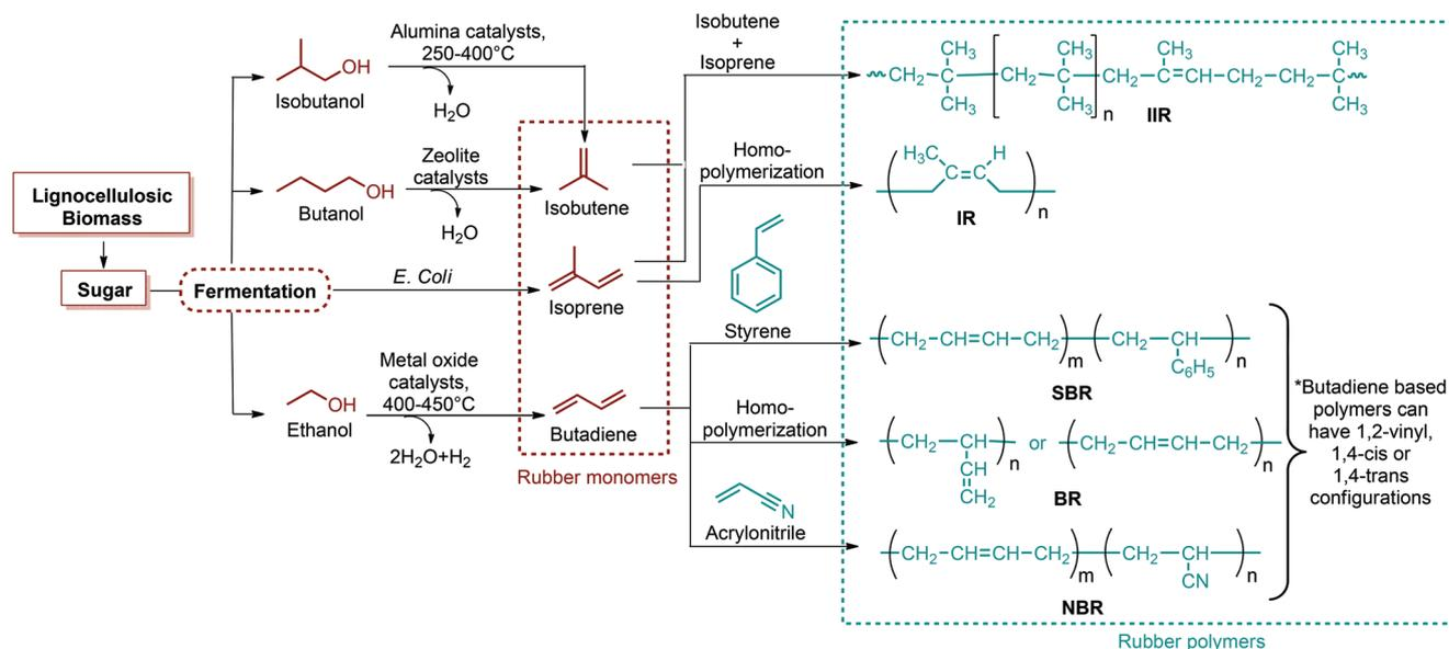
Fig. 39 Lignocellulosic biomass derivable rubber monomers and polymers.
