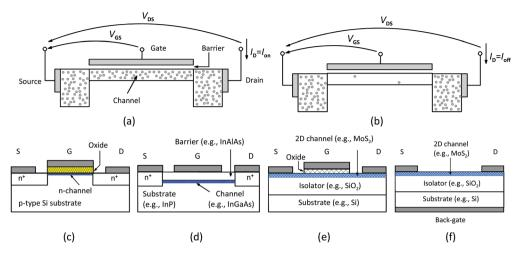
Fig. 4 Basic FET structures. Generic structure of a FET (a) in the on-state and (b) in the off-state. (c) Conventional Si n-channel MOSFET. (d) HEMT. (e) 2D MOSFET. (f) Back-gate 2D MOSFET frequently used for proof-of-concept purposes. Note that HEMTs and 2D MOSFETs do not possess pn junctions as present in conventional Si MOSFETs shown in (c) but rather resemble the junctionless MOSFET which is intensively investigated at present.<sup>42</sup>
