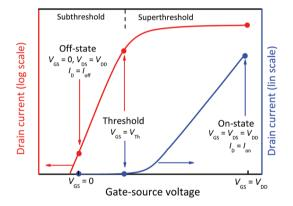
**Fig. 5** Transfer characteristics of an n-channel FET showing the drain current  $I_D$  as a function of the gate-source voltage  $V_{\rm GS}$  together with the on and off operating points for CMOS logic. Note that the scale of the left current axis is logarithmic and that of the right current axis is linear.
