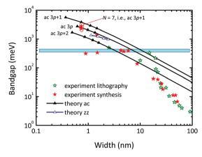
Fig. 9 Bandgap of GNRs vs. ribbon width. Shown are theoretical data obtained by the GW method for ac (armchair) GNRs of the 3p, 3p + 1, and 3p + 2 families (full triangles and lines, p is an integer) and for zz (zigzag) GNRs from ref. 87, together with measured results for chemically synthesized<sup>89,90,95</sup> and lithographically patterned<sup>93,94</sup> GNRs.
