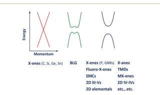
**Fig. 7** Schematic band structure of 2D materials relevant for transistors. BLG: bilayer graphene; GNR: graphene nanoribbon; TMD: transition metal dichalcogenide; SMC: semimetal chalcogenide.
