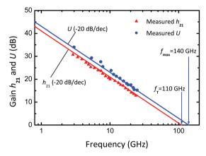
Fig. 6 Small-signal current gain  $h_{21}$  and unilateral power gain U of a RF FET as a function of frequency, after ref. 43 and 44. The characteristic frequencies  $f_{\rm T}$  and  $f_{\rm max}$  are obtained by extrapolating the measured  $h_{21}$  and U with the characteristic slope of -20 dB per dec.
