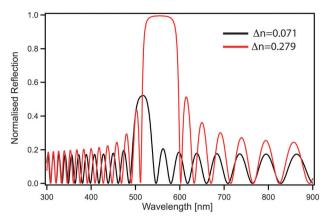
**Fig. 9** Refractive index dependence of one-dimensional stacks. The black line shows the calculated spectrum of a multilayer stack composed of 40 alternating 70 nm thick PS and PI layers (typical values for block copolymer based multilayers) obtained by the transfer matrix method. The red line corresponds to a multilayer stack with the same layer dimensions, where the PS layers are replaced by quanine.
