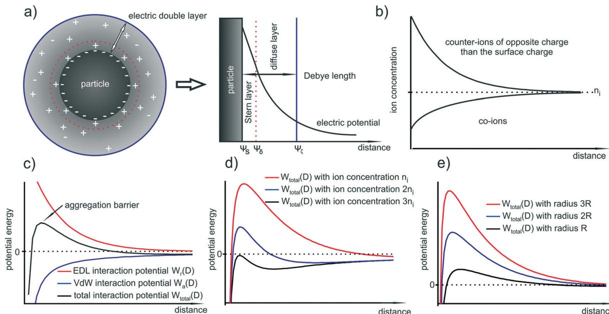
**Fig. 2** (a) Formed electrical double layer (EDL) around a NP due to the Gouy–Chapman model which consists of the inner Stern layer and the outer diffuse layer (b) corresponding decrease in the counter- and co-ion concentrations with respect to the distance from the particle surface; (c) schematic of the EDL, van der Waals and total interaction potentials (TIP) of two NPs; (d) and (e) influence of the ion concentration and the particle size on the TIP.
