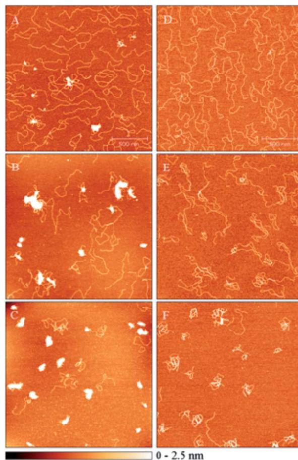
**Fig. 3** AFM images of linear plasmid pSP73 (2464 bp) mixed with flexicates at various DNA base : flexicate ratios. (A–C) DNA with Δ-Fe<sub>2</sub>L<sup>1a</sup>]<sub>3</sub>Cl<sub>4</sub> at 5 : 1, 3 : 1 and 2 : 1 ratios, respectively. (D–F) DNA with Δ-Fe<sub>2</sub>L<sup>2a</sup>]<sub>3</sub>Cl<sub>4</sub> at 1 : 2, 1 : 4 and 1 : 6 ratios, respectively.
