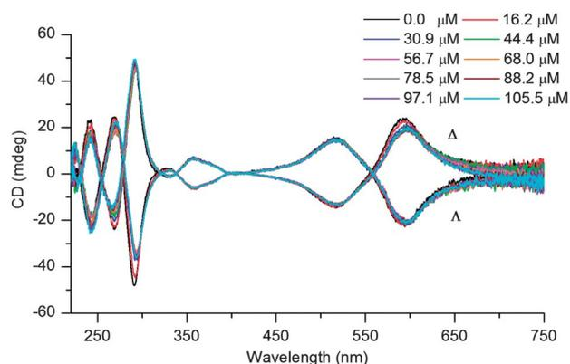
**Fig. 4** CD titration series for Δ-Fe<sub>2</sub>L<sup>1a</sup>]<sub>3</sub>Cl<sub>4</sub> at constant flexicate concentrations (15 μM) and increasing ct-DNA concentrations (indicated in legend). TRIZMA® base buffer (1 mM, pH 7.2). Path length 1.0 cm.
