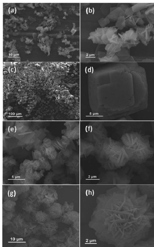
Fig. 1 SEM images of the synthesized NiCo<sub>2</sub>O<sub>4</sub> samples from different hydrothermal reaction times: (a–b) 3 h; (c–d) 6 h; (e–f) 9 h; (g–h) 12 h.
